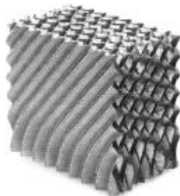
Figure 1. Photograph of a segment of the high-capacity packing B1-250M
