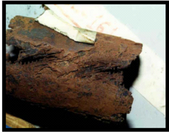
Figure 12 – Note the V Shaped Corrosion Damage which is Common on all Completions and in Every Joint
