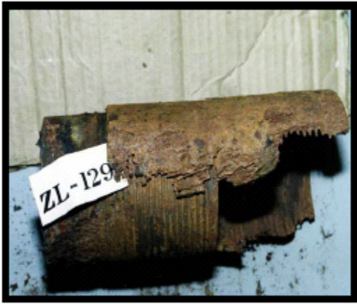
Figure 12 – Note the V Shaped Corrosion Damage which is Common on all Completions and in Every Joint
