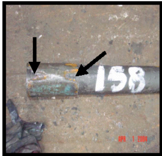
Figure 13 – V Shaped Damage to the Tubing Box in ZK-152 – see arrows
