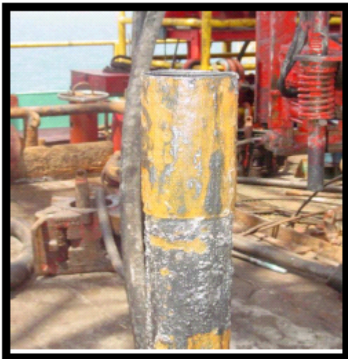
Figure 13 – V Shaped Damage to the Tubing Box in ZK-152 – see arrows
